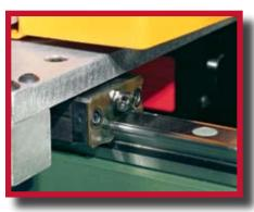
Saw tables glide on precision-finished rails and linear bearings to ensure smooth travel and increased bearing life.
