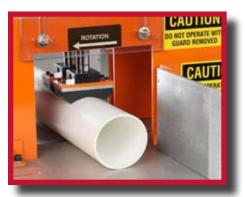
Up-Cut Saws feature positive clamping for superior cut quality.
