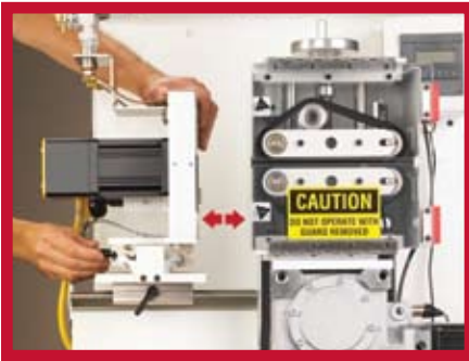
On both models, the cutter moves laterally for easy string-up.
