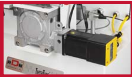
Servo gearbox reduces backlash and increases efficiency.
