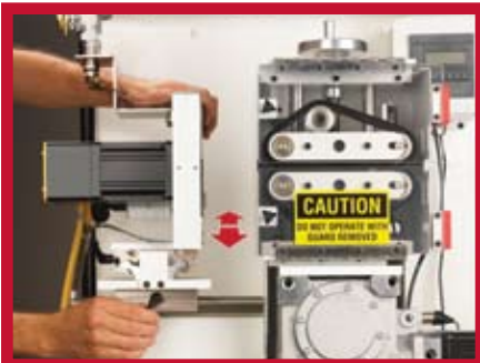
The IC-5 cutter can be moved to either side of the belt, potentially increasing belt life dramatically, and out of the way for coiling.
